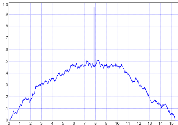
Figure 21. The dependence of the correlator output signal on the phase tuning (relative units)
